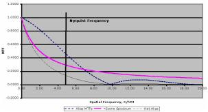
**Figure 1.** A "typical" scene spectrum cascaded with the MTFs of the camera lens, optical pre-filter and sensor.
